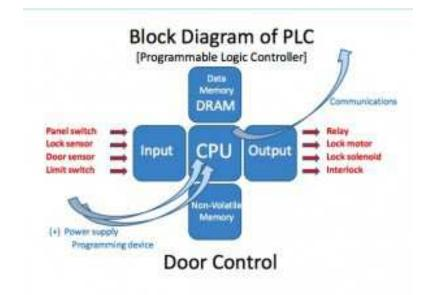
Diagram showing the typical parts of a PLC used for door-control systems. Image courtesy of Teague Newman
